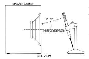
Slight off-axis positioning will minimize stressing the ribbon on loud sound sources.
