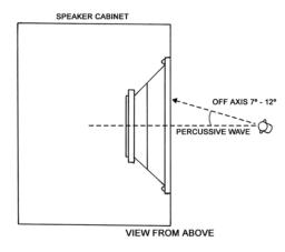
Angling the microphone slightly will minimize stressing the ribbon. Due to the microphone's pickup pattern, sound will not be affected.
